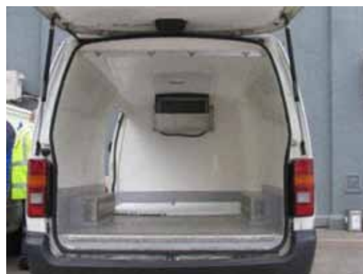
FIGURE 4 Inside of a truck with a transport refrigerating system
