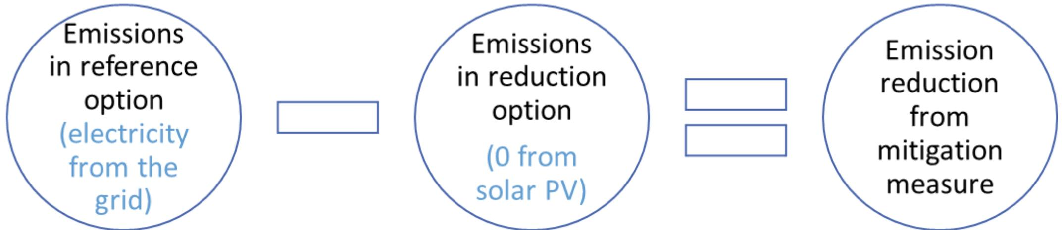
$$Emissions_{reference\ option}(t\ CO_2) = Electricity_{solar\ PV}(MWh) \times Grid\ Emission\ Factor\left(\frac{tCO_2}{MWh}\right)$$
