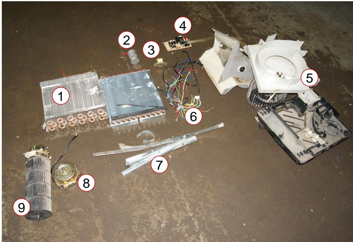
1. Aluminium-copper heat exchanger
